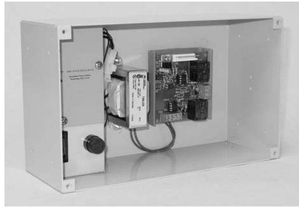
The Remote Monitoring Station features a time delay “ON” circuit that is field settable from 0 to 5 minutes. The unit can be used to prevent incidental or unintentional alarm notification due to inadvertent activation of an emergency shower or other monitored device.
